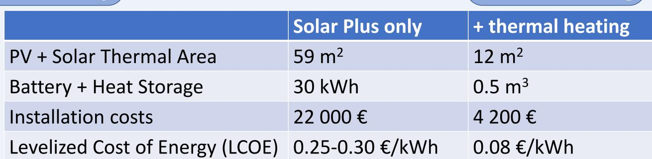
Thermal heating and storage installation is quite cheaper and less complex compared to PV/Solar Plus. However, heating alone cannot fulfil all domestic energy needs therefore some mixture is necessary.
